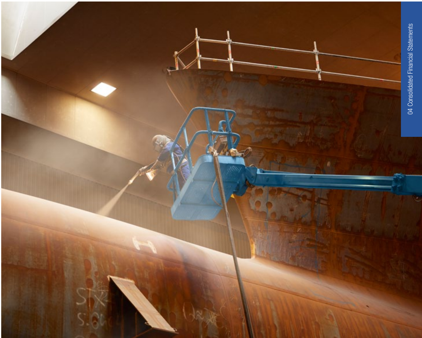
Blasting work on the bow of a cruise ship in Saint-Nazaire, France
